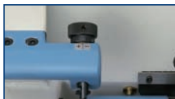
2 Trace point with micrometric adjustment.
